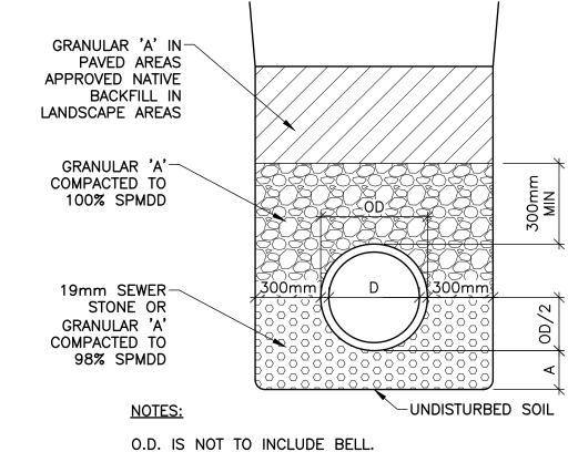
O.D. IS NOT TO INCLUDE BELL. A = D/4 BUT NOT LESS THAN 150mm
