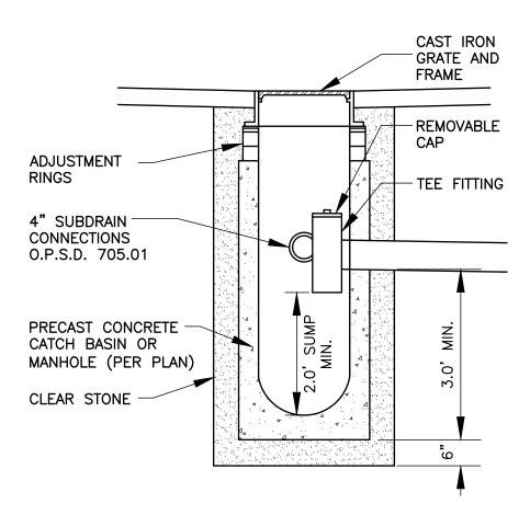
T-Y TRAP AND OUTLET CONTROL NOT TO SCALE
